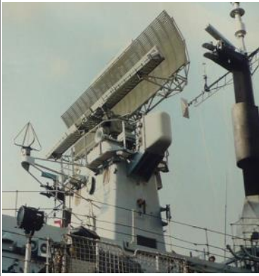
Type 670 Jammer Port Radome below the Type 1022 Radar fitted on a Type 42 Destroyer
