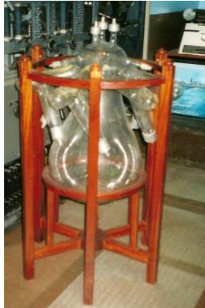
A Mercury Arc Rectifier housed in a display frame
